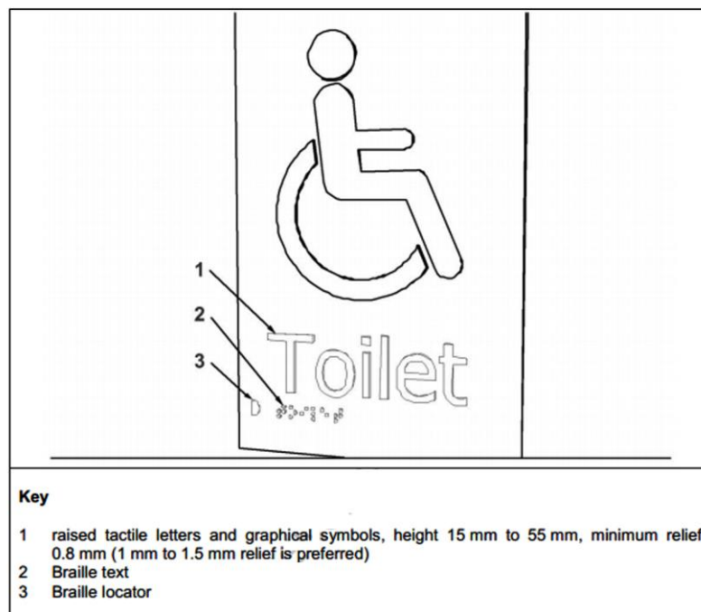
Figure 88: Details of raised tactile sign dan Braille
